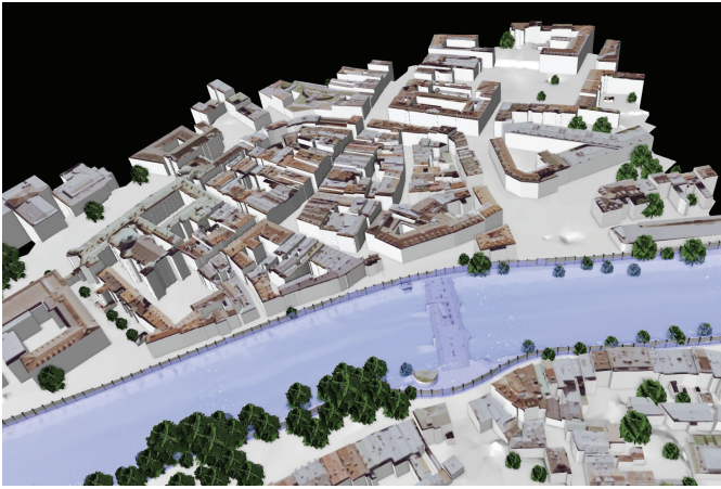
Fig. 4. City protected by mobile walls. The user has drawn barriers on each side of the river. The simulation of rising water levels confirms the robustness of the chosen design.
