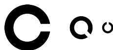
Figure 3.1: Landolt C , or Landolt ring , with a gap at one of eight possible positions: top, bottom, left, right, or 45° in between.
