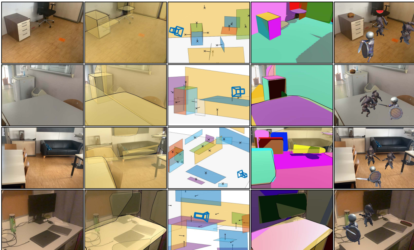
Fig. 15: Indoor localization examples for AR applications on mobile devices leveraging AR Foundation capabilities. First column: RGB image of the scene. Second column: Detected planes. Third column: Estimated camera pose in the model coordinate system. Fourth column: Registered parametric model planes to planes detected in the scene. Fifth column: Registered virtual objects.
